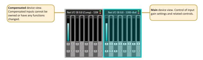
The compensated output's level is controlled in the stagebox itself, so any Dante device can receive the compensated signal, it does not have to be an SSL console.
